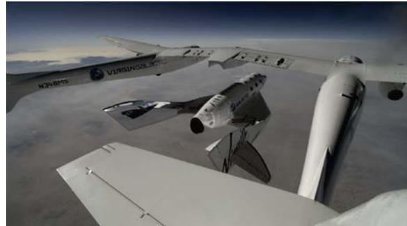
Figure 1: SpaceShipTwo release from WhiteKnightTwo
