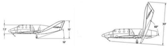
Figure 2: Normal and feathered configuration
